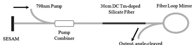
Fig. 3. Schematic of mode-locked Tm-doped silicate fiber laser.
