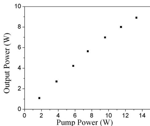
Fig. 1. Laser output power versus the absorbed pump power of the 20-cm-long Tm-doped silicate fiber (with a core diameter of 18  $\mu\text{m}$ ) laser.
