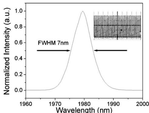
Fig. 4. Laser spectrum of mode-locked Tm-doped silicate fiber laser. Inset, pulse train of the mode-locked laser.
