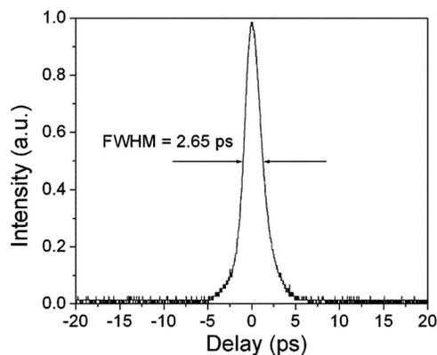
Fig. 5. Intensity autocorrelation of mode-locked Tm-doped silicate fiber laser at 10 mW output.
