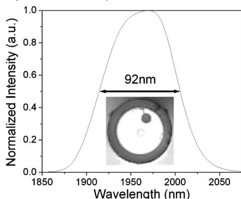
Fig. 2. ASE spectrum of Tm-doped silicate glass fiber. Inset, microscope image of the fiber cross section.
