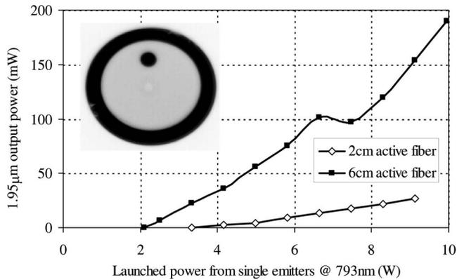
Fig. 1. 1950 nm laser output versus launched multimode pump power at 793 nm in a cladding-pumped short-cavity DBR fiber laser. Inset, microscopic image of the active fiber.
