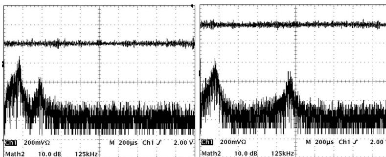
Fig. 4. Intensity of the DBR fiber laser and its FFT spectrum at two different pump powers. Left, 340 mW pump power; right, 550 mW pump power.
