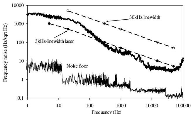
Fig. 5. Frequency noise spectrum of the DBR fiber laser, as compared with noise floor and the published data [5].
