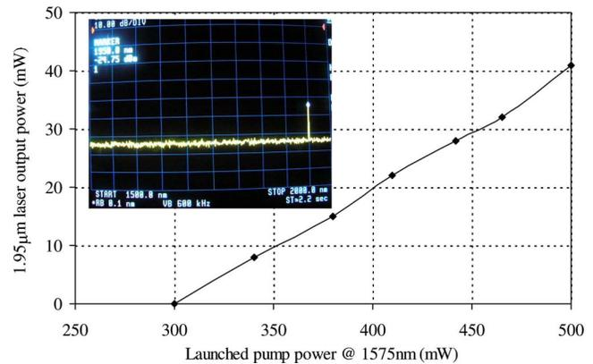
Fig. 2. (Color online) 1950 nm laser output versus launched single-mode pump power at 1575 nm in a core-pumped short-cavity DBR fiber laser. Inset, spectrum of the DBR fiber laser.
