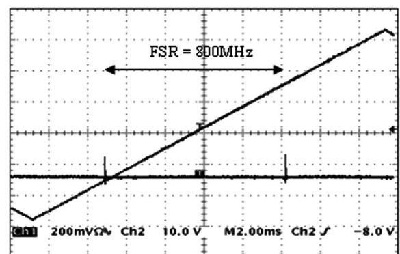
Fig. 3. Scanning spectrum of the fiber Fabry–Perot interferometer.
